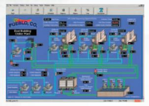
The CH530 controller features the Adaptive Control microprocessor, which has the ability to keep the chiller online, producing reliable cold water during extreme operating conditions when other chillers would usually trip off.
